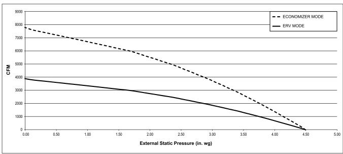
Fig. 15 - 50HC\*\*20 Supply and Exhaust Fan Performance Curves
