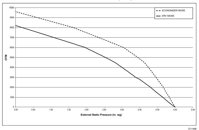
Fig. 16 - 50HC\*\*24 Supply and Exhaust Fan Performance Curves
