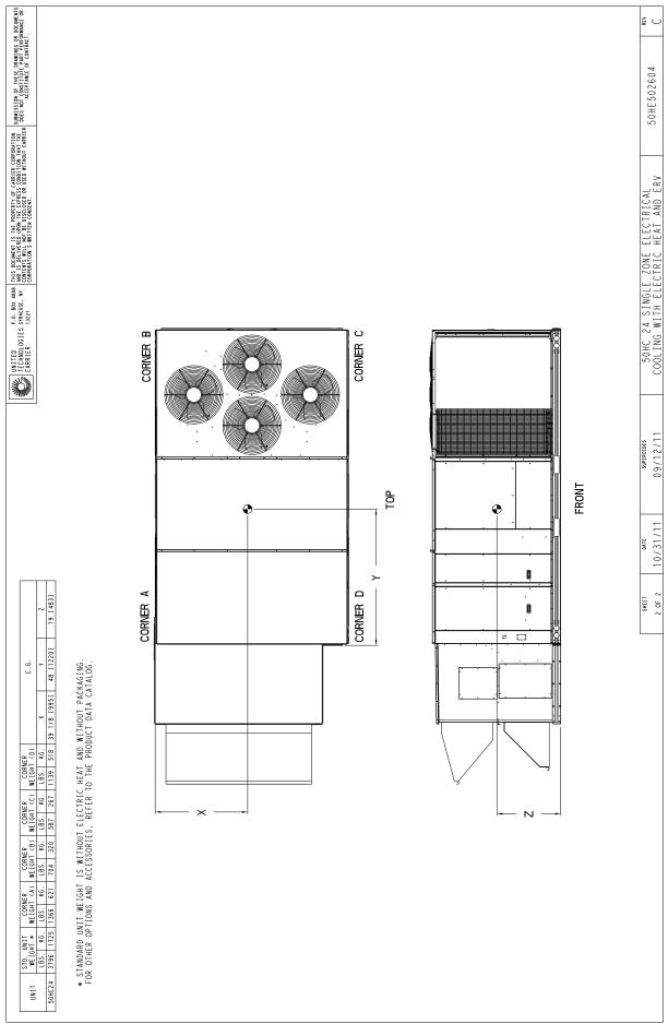
Fig. 6 - 50HC-24 Single Zone Electric Cooling with Electric Heat and ERV (Sheet 2 of 2)
