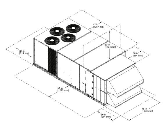
Fig. 10 - Clearances for ERV on Size 24 & 28 Base Units
