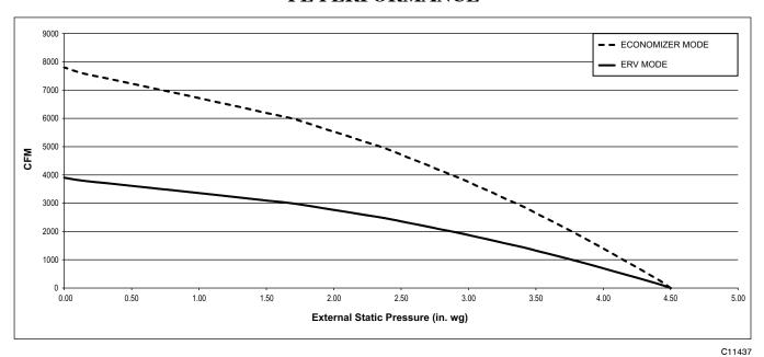
Fig. 14 - 50HC\*\*17 Supply and Exhaust Fan Performance Curves
