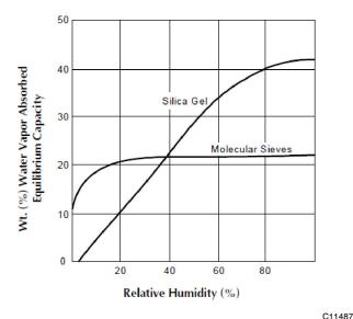
Fig. 21 - Effect of Relative Humidity on Desiccant Capacity
