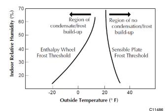
Fig. 22 - Frost Threshold comparison
