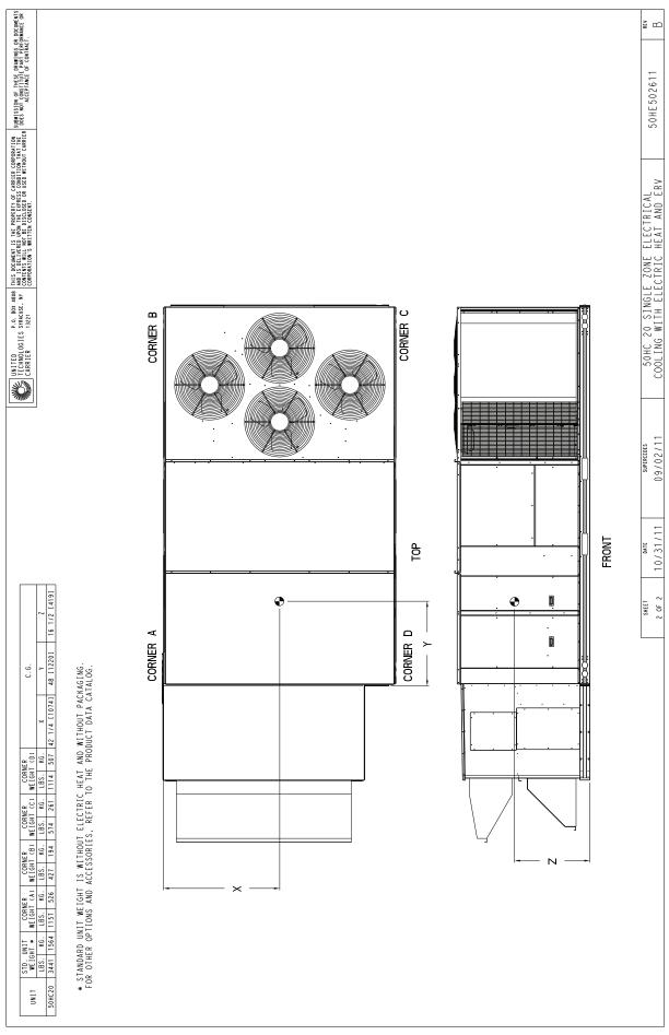
Fig. 4 - 50HC-20 Single Zone Electric Cooling with Electric Heat and ERV (Sheet 2 of 2)
